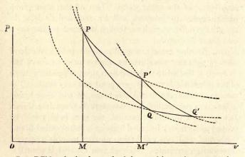
Let PP' be the isothermal of the working substance at the temperature  $t_i$ , of the hot body; QQ' that at the temperature  $t_o$  of the cold body; while QP and P'Q' are the adiabatics of the first and third operations respectively. Also
